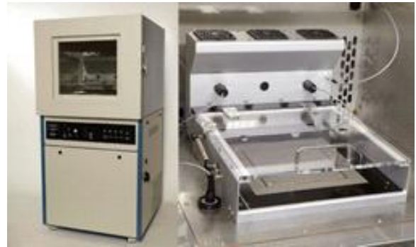
<Figure 1> Sweating guarded hotplate integrated system (SGHO-8.2)
