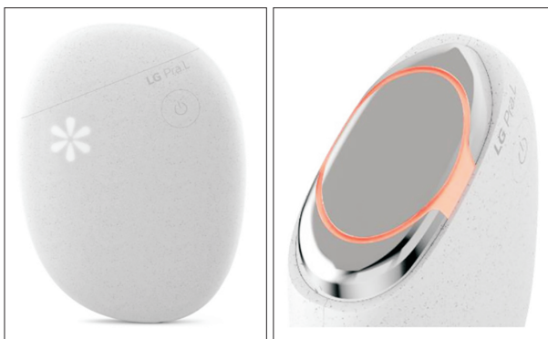
Fig. 1. Combined application of two techniques—electroporation (EP) and low-frequency sonophoresis (SP)—using a BBS1 device (LG Electronics). Simultaneous application of EP with SP physically creates transient new aqueous pathways (pores) in the stratum corneum, which enhance skin permeation. Maximizing absorption of active ingredients is achieved by repeating these treatments at an efficient rate.
