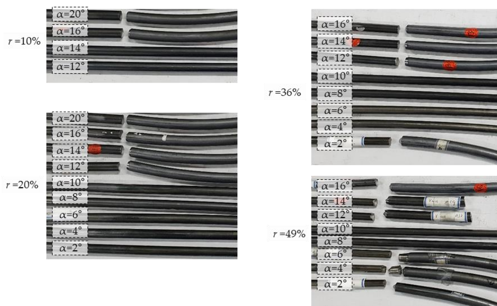
Figure 2. Fractured and non-fractured specimens for various r and \alpha combinations. Thirteen specimens were not fractured, while sixteen specimens were fractured.
