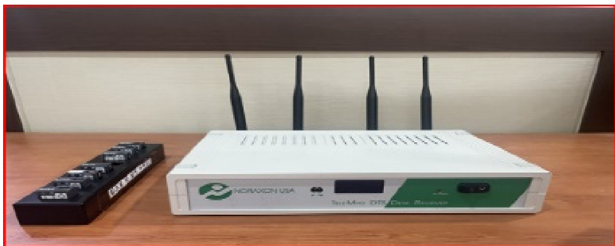
Figure 3. Electromyography device (Telemyo-DTS, NORAXON, USA).
