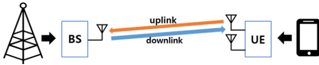
FIGURE 1. The 1 \times 2 SFLC-OFDM system model.
