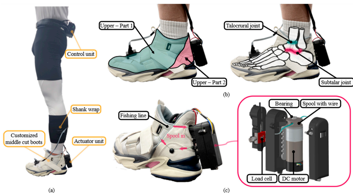
Figure 2. (a) Configuration of AVC-Shoes. (b) Design of upper part of AVC-Shoes, which is divided into two parts to generate a firm compression force on the talocrural and subtalar joints. (c) Design of actuation component. Spooling the fishing line generates a compression force on the ankle joint along the wire path (right inset: complete configuration of the actuator unit).
