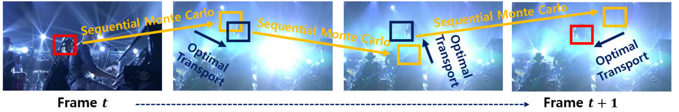
FIGURE 2. Pipeline of the Proposed SOTA Tracker. Given the target's configuration at the current frame t , the seamless mapping module of the proposed tracker approximates its configuration at the next frame t + 1 via sequential Monte Carlo sampling explained in Section III-B. Subsequently, the exact mapping module refines this approximated configuration by optimally adjusting it using the optimal transport technique described in Section III-A. This process iterates multiple times to accurately determine the target's configuration at the next frame t + 1 , as illustrated in Section III-C.
