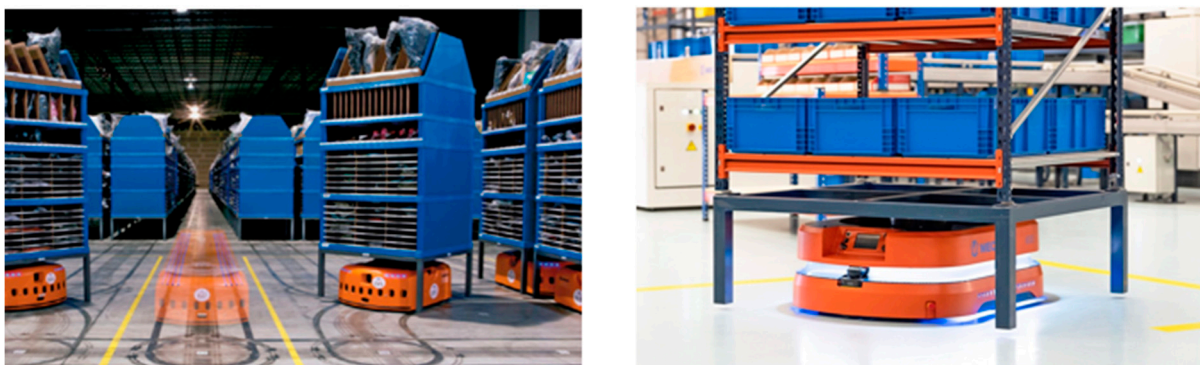
Top row: Automated Guided Vehicle, Autonomous Mobile Robot Source from CLO, Mecalux
