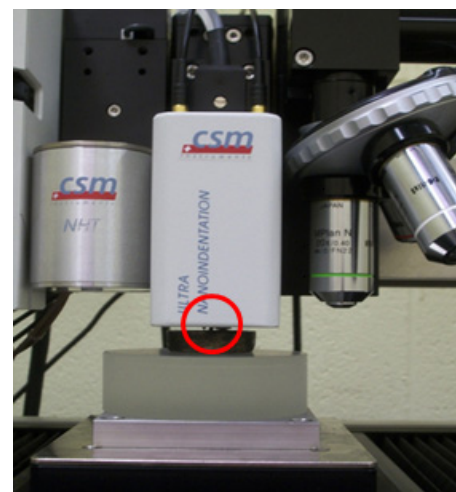
Fig. 1 Picture of the nanoindentation instrument and a specimen installed
