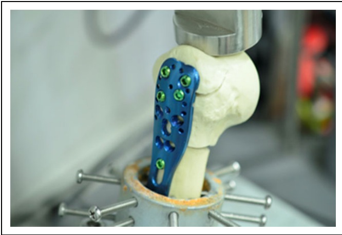
Figure 4. Structural failure as a failure mode as shown in the 4-screw group.
