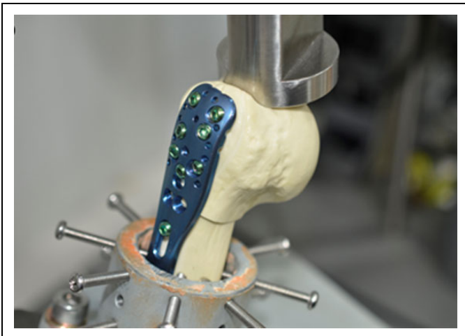
Figure 5. Interfragmentary gap closure as a failure mode as shown in the 7-screw group.
