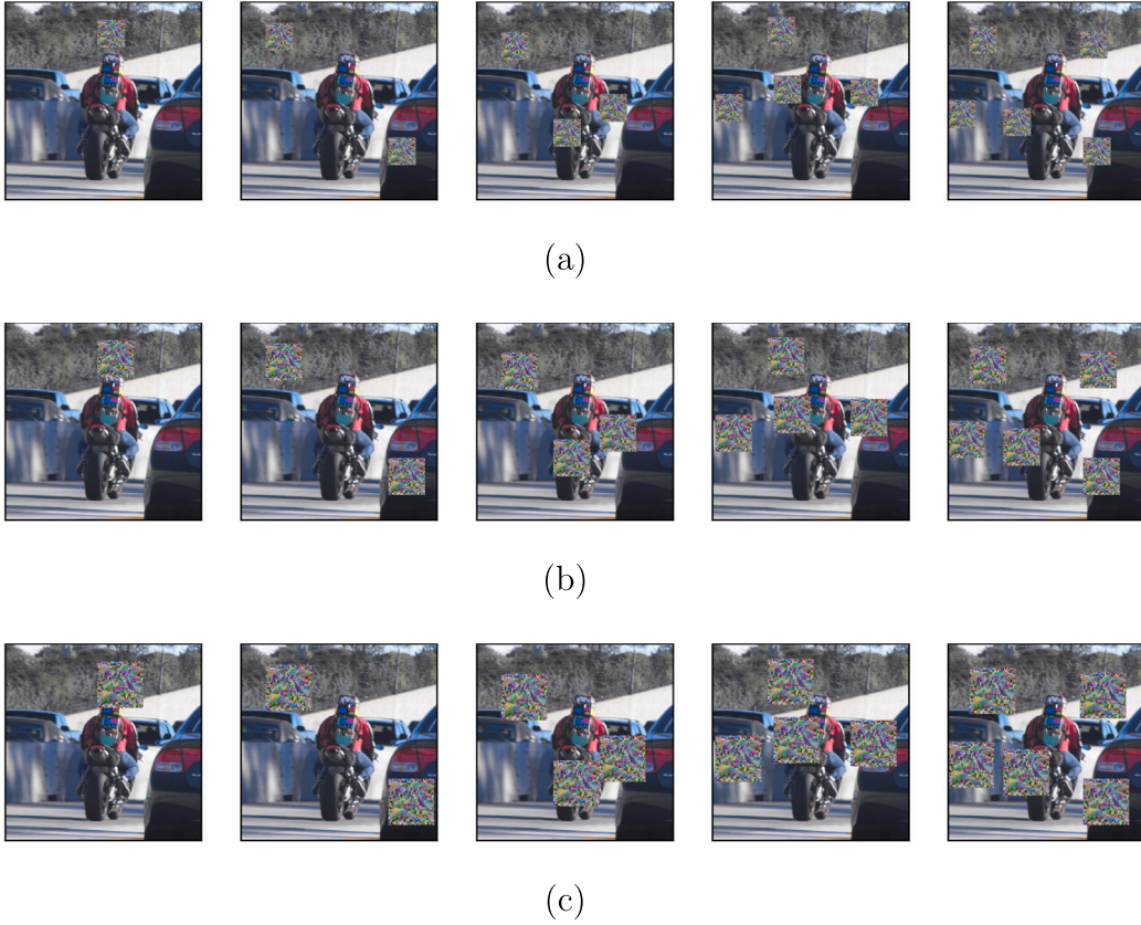
Fig. 6. (a), (b), and (c) represent Dpatch sizes S, M, and L, respectively, while the number of adversarial patches ranges from 1 (left) to 5 (right), gradually increasing. When the patch size is large (c), it occupies a relatively wide area of the entire image. As a result, the overall CPV value for the image region increases, leading to instances where the patch area is not accurately detected.
