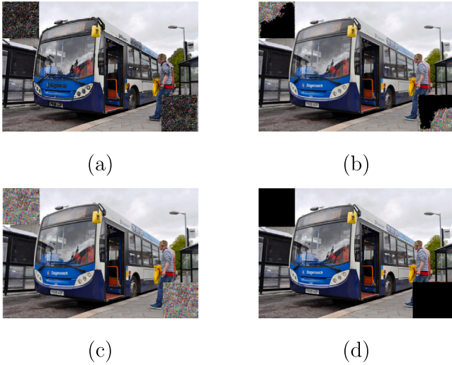
Fig. 8. When subjected to a Dpatch attack, (a) LGS (Naseer et al., 2019) shows that not only the patch but also the area around the patch is affected; (b) SAC (Liu et al., 2022) indicates that when there are two patches, the defense is not effective; (c) Jedi (Tarchoun et al., 2023) shows that defense is possible depending on the threshold, so it fails without proper adjustment. (d) Our methodology, RAPID, detects and masks the patches effectively.
