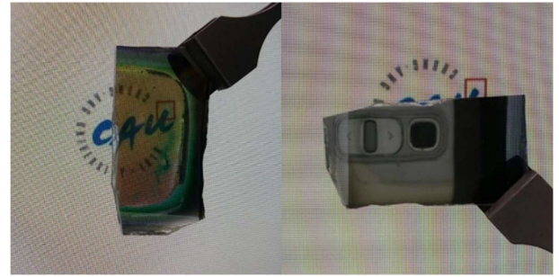
Fig. 3. Photograph image of fabricated wire-grid polarizer with glass molded nanograting structure on LCD monitor.
